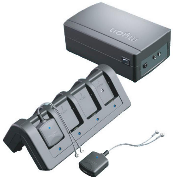
Not only does this make the system very reliable and easy to use, it also means that the time it takes from the signals are recorded until they are forwarded from the receiver is a constant 16 milliseconds. The fact that it is constant is essential when synchronizing with other equipment, the fact that it is low is crucial if you want real-time feedback.
